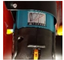
Speed selector is located on the motor
