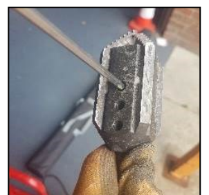
Trim back damaged Shaft
