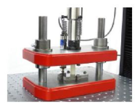
A sample of the product at approximately .25-inches is laid flat and a machine pushes down on the specimen until it begins to compress. The PSI it requires to sheer the sample is its "Compression Strength". The amount it swells when the pressure is applied is also measured.
