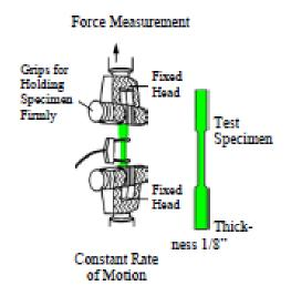
A piece of finished product, with a maximum thickness of .125-inches, is machined into a dog-bone shape. Each end of the test specimen is placed in opposite facing clamps which then attempt to pull it apart.
