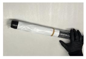
• Copy the Off Limits Zone measurement and mark on the surface of the Calibration Tube using a marker pen.
