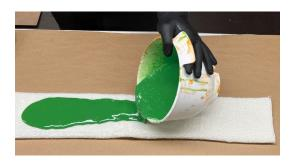
Apply resin in portions and work it thoroughly into the material.
