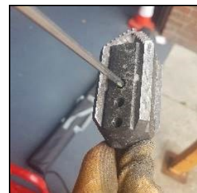
Trim back damaged Shaft
