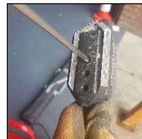
Trim back damaged Shaft
