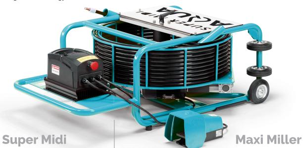
A high-speed multi-use machine. For cleaning and descaling 3-6" pipes and brush coating 2-8" pipes. 110v model. 1/2" Shaft with thin outer casing making it safe for the operator to hold. Operator presence control, electric safety clutch and E-Stop for added safety. Range 65ft or 97ft by adding a 32ft extension.
