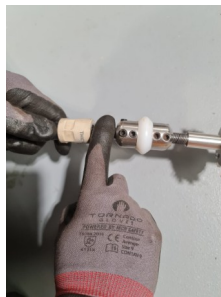
Leave a gap between the sleeve and the Smart Spider / Smart Sweeper of approximately 6mm (1/4").
