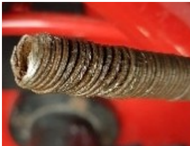
Damaged Shaft. Needs to be trimmed.
