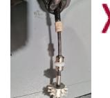
Leave a gap between the sleeve and the Smart Cutter™ Hub of approximately 6mm (1/4").
